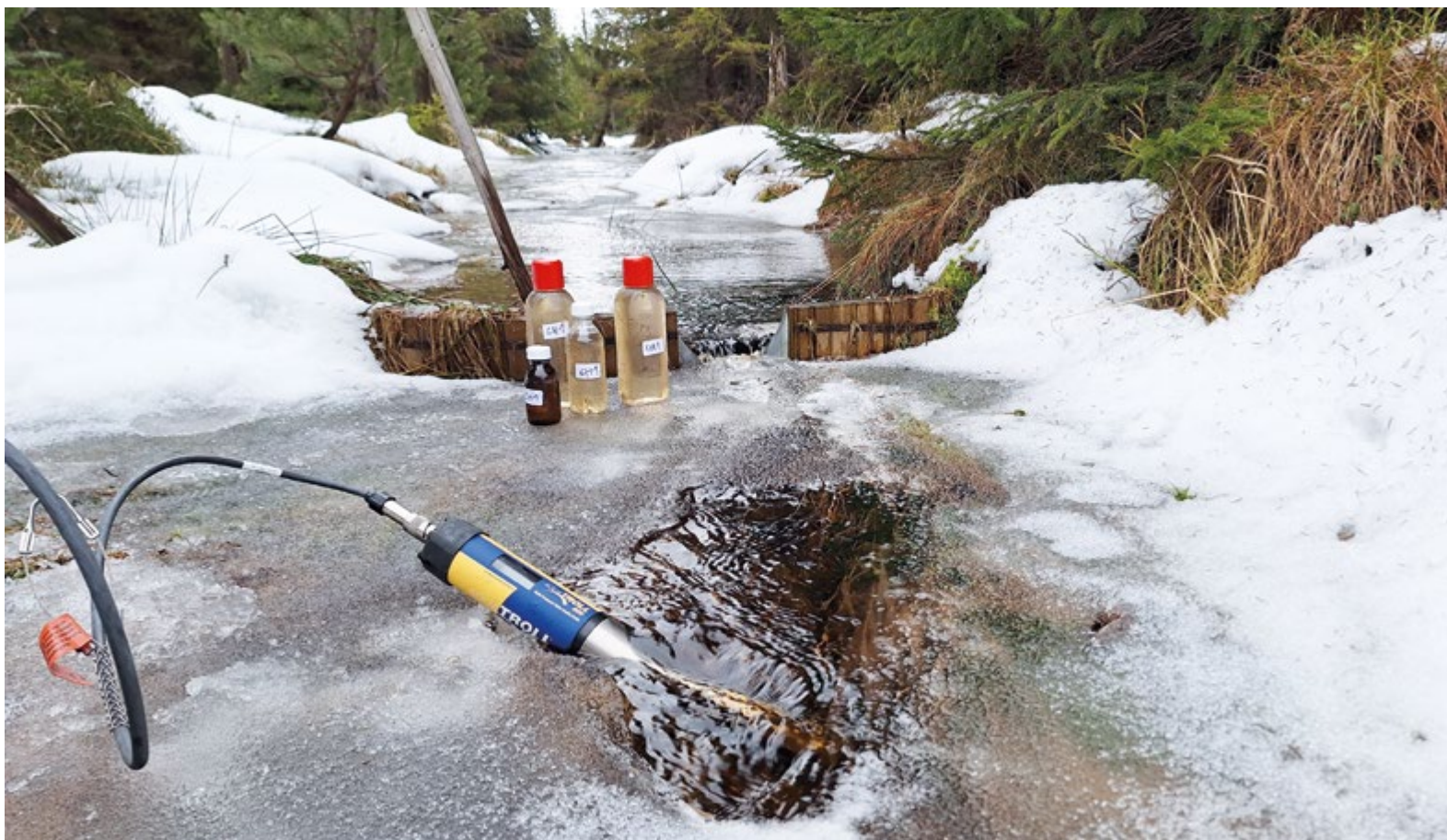
Fig. 6. Sampling and measurement of chemical parameters of surface waters at profile V7-CH1
