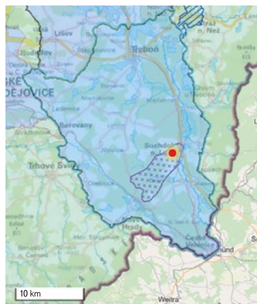
Fig. 4. Catchment area (purple marked area) of groundwater abstraction ČEVAK Suchdol n/Lužnicí (ID Surová voda : 11300600) on the basis of the Progeo, s. r. o., hydraulic model and its inclusion in the broader context of the relevant hydrogeological district
