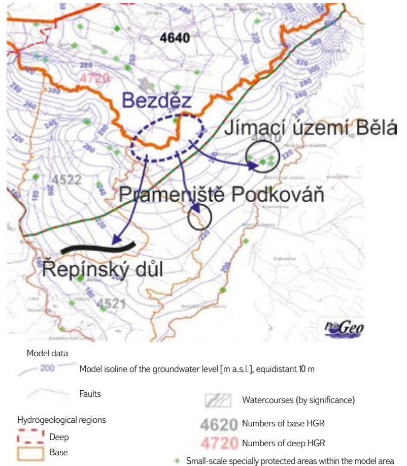
Fig. 11. Model isolines of the groundwater level from a model from PROGEO, s. r. o., with marking of the probable location of infiltration of low-tritium waters (blue oval) and the direction of water flow (blue arrows). Modified after [1]
