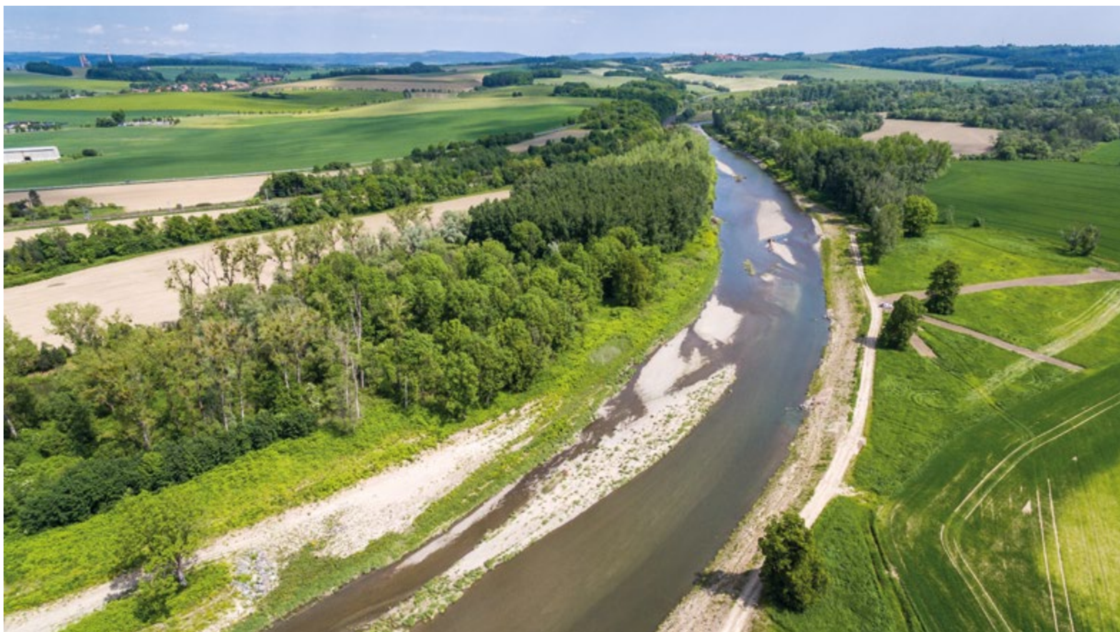
Fig. 3. Widening of the Bečva river allowed the creation of gravel bars (Source: Morava River Basin Management)
