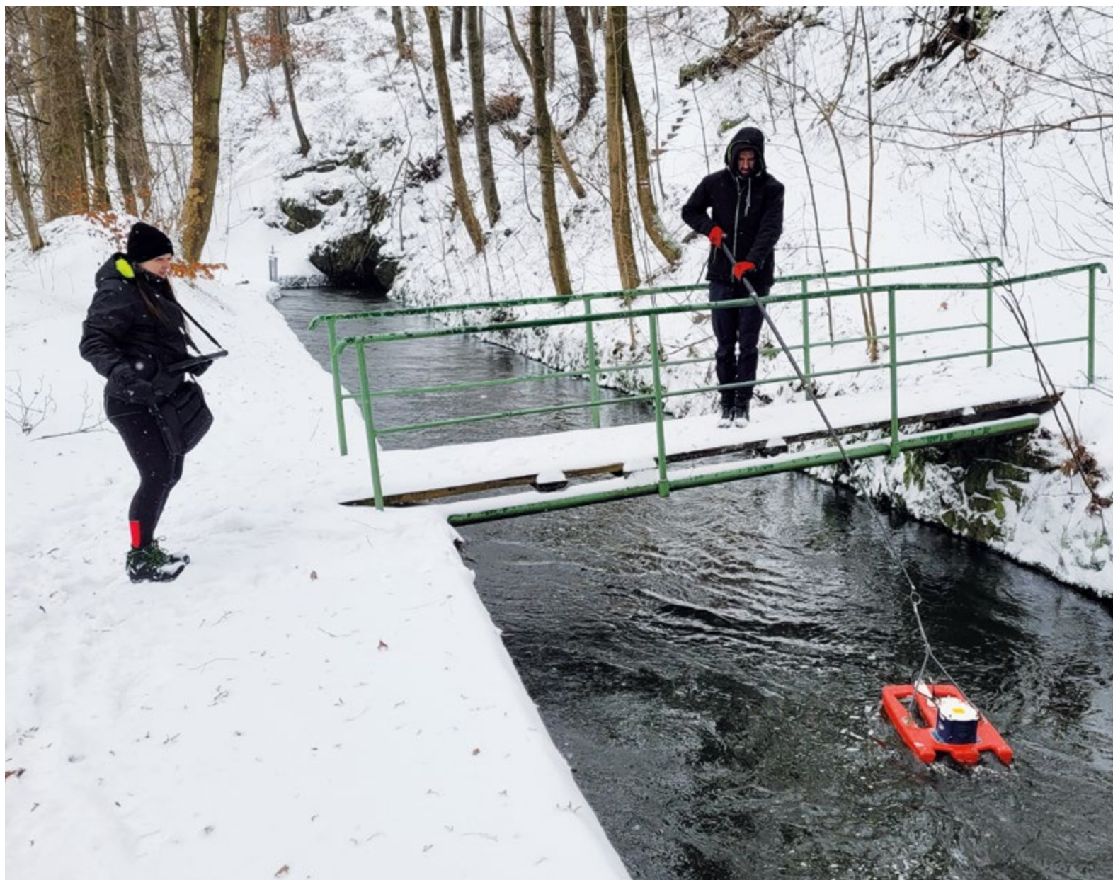
Fig. 1. Discharge measurement using ADCP RDI StreamPro, Weissshuhn flume in Žimrovice, 8th January 2024 (Photo: J. Unucka)
