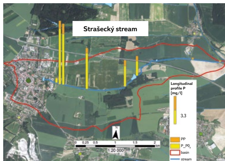
Fig. 1. An example of a significant change in phosphorus concentrations in the longitudinal profile downstream from Nové Strašecí (5,500 inhab.) on November 10, 2015, when 95 % of the flow in the Strašecký stream (5.0 km) consisted of WWTP discharge. Total phosphorus concentration decreased slightly from 7.4 mg/l in the WWTP outlet to 3.1 mg/l and 2.3 mg/l above and below Konopas pond, respectively, which was drained completely at the time. In the lower part of the stream, retention was significant and the concentration dropped to 0.210 mg/l at the confluence with Loděnice river. Particulate phosphorus (PP) is the difference between total and dissolved reactive phosphorus ( PO_4 -P)
