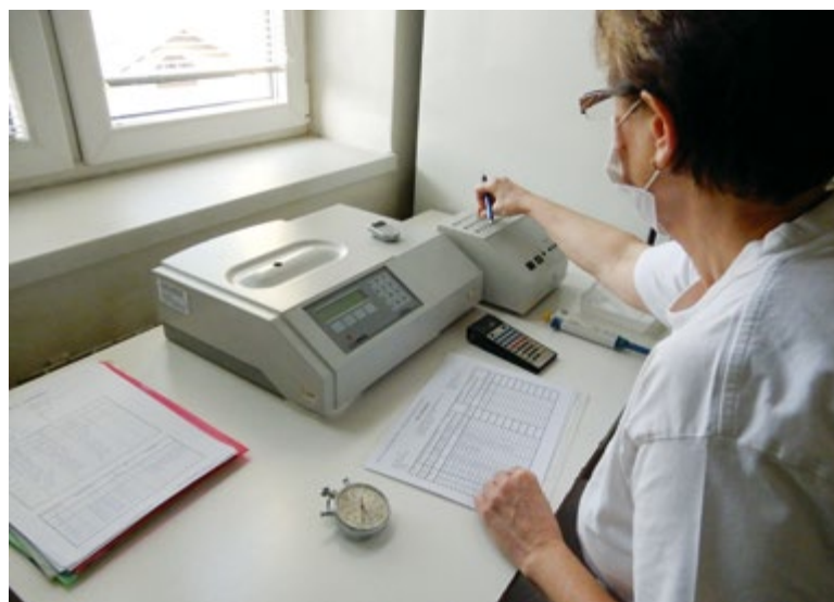
Fig. 3. Measurement of luminescence intensity changes during the test
