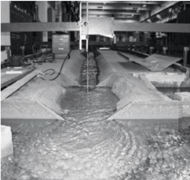
Fig. 2. Full space model of the channel in the transition zone of scour hole development (left); symmetric half-space model of the channel with axis at the flume glass wall (right) – all under laboratory conditions
