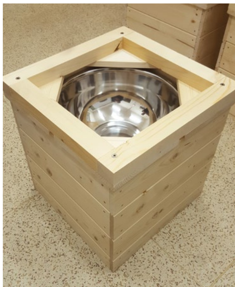
Fig. 4. Rain gauge for precipitation capture for PAH analysis
