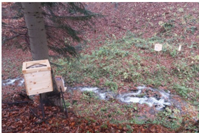
Fig. 5. Rain gauges for capturing bulk and throughfall precipitations at the Bystřice site (5th November 2020)
