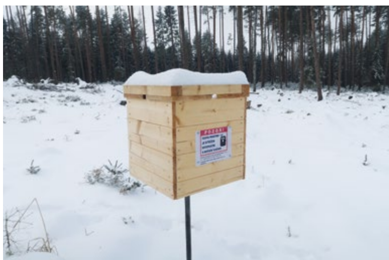
Fig. 6. Rain gauge for capturing bulk precipitation at the Košetice site (8th February 2021)
