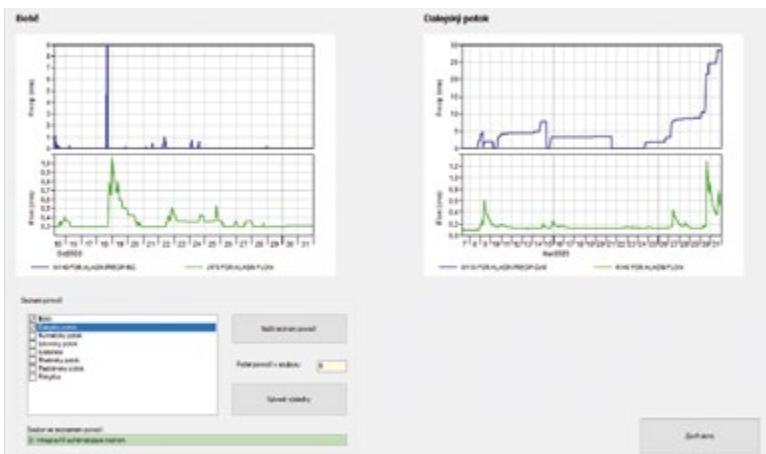
Fig. 3. Window for the result viewing of HEC-HMS simulations for the decision making
