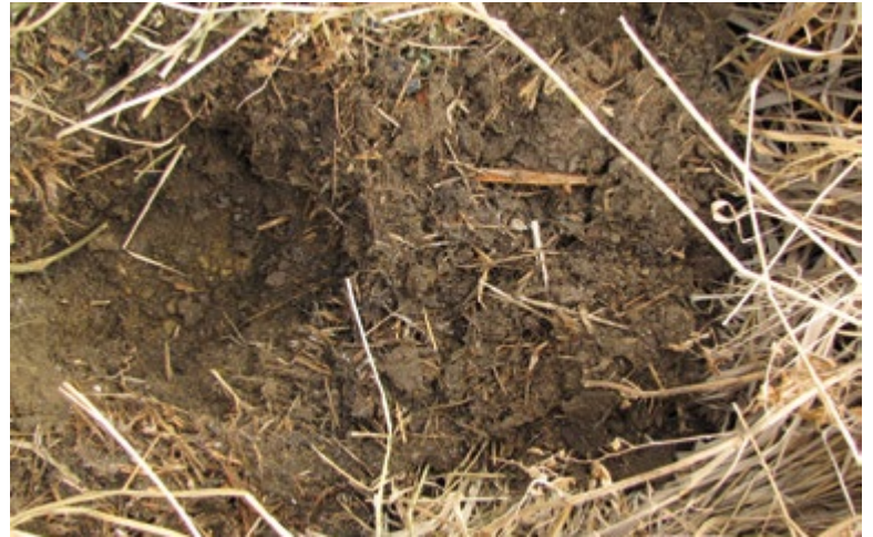
Fig. 4. Structure of the dewatered and stabilized mixture of sludge and wetland vegetation after 7 years of operation of the STRB unit and after shutdown for one season to complete the process of stabilization and sanitation of the mixture
