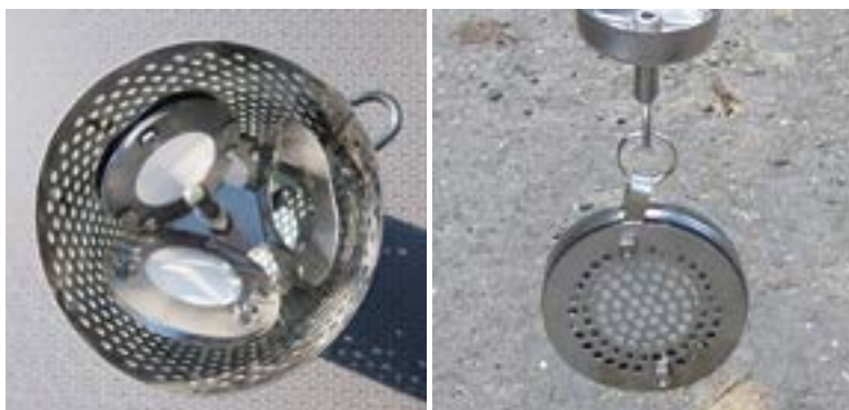
Fig. 5. Passive sampler POCIS in big canister (left) and in the casing (right)
