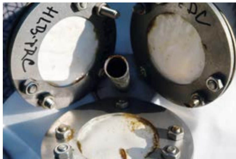
Fig. 6. Exposed passive samplers POCIS
