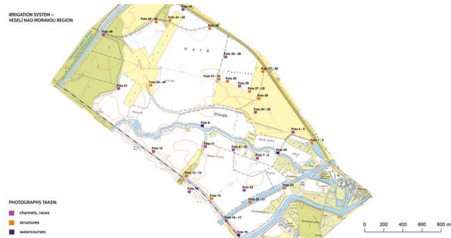
Fig. 2. Example of location processing of individual objects and selected important elements of the irrigation system in the surroundings of Veselí nad Moravou on the basis of current field investigations, ZABAGED® data
