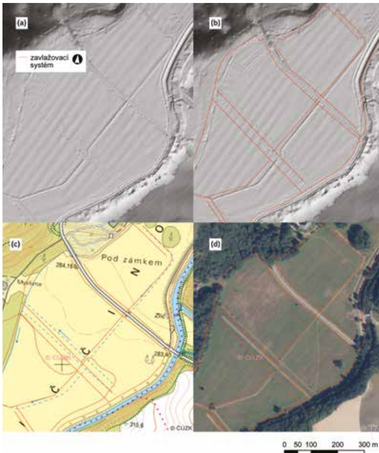
Fig. 5. Example of differentiation of the remnants of meadow irrigation by furrows and channels in the Úpa river floodplain above Česká Skalice. Demonstration of the use of the TIN DTM at the site to determine the location of the individual parts of the irrigation system: (a) TIN DTM; (b) TIN DTM, indicating the course of the irrigation system (in red); (c) extract of the basic 1 : 10,000 map, indicating the course of the irrigation system; (d) aerial image extract, indicating the course of the irrigation system. ZABAGED® data
