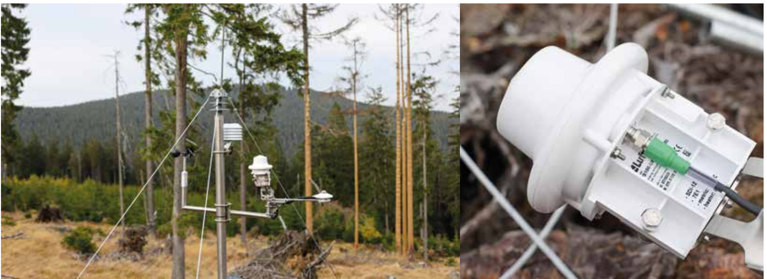
Fig. 1. View of the radar rain gauge installation and detail of the WS100 sensor
