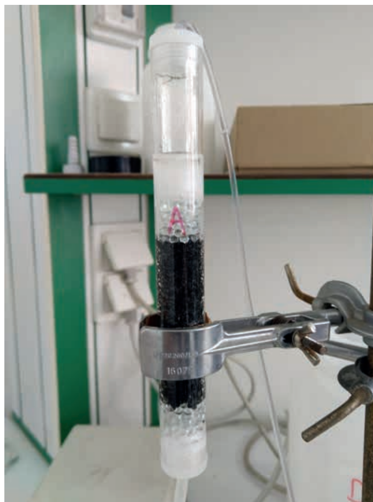
Fig. 2. Photo of glass column filled with GAC during the testing (author: Anna Kólová)
