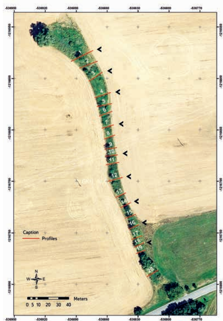
Fig. 3. Location of the 20 transverse profiles in the gully erosion: the black arrow shows 9 selected profiles (base map: GKÚ Bratislava, NLC, 2019)
