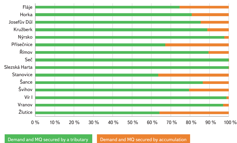
Fig. 8. Use of water accumulation in the storage space of water reservoirs for the security of current water demand and minimum discharges in the HadGEM2 scenario
