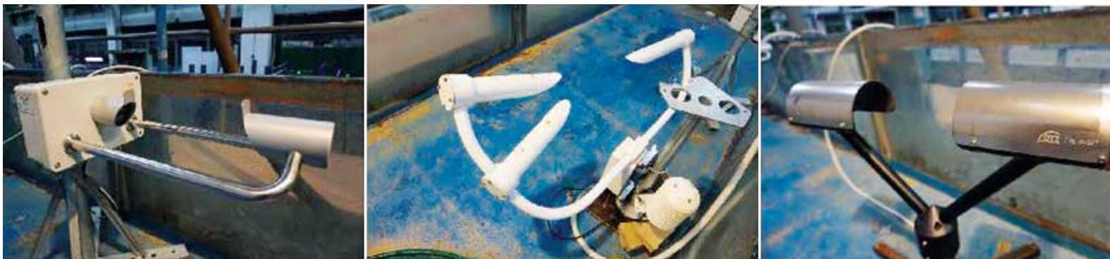
Obr. 1. Disdrometry zleva: Thies LPM, PWS100, Parsivel
