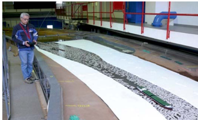
Obr. 5. Plavba MNL 11600 proti proudu Fig. 5. Up-stream navigation of cargo ship type MNL 11600
